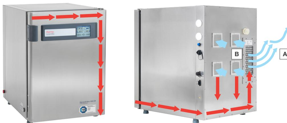
**Figure 2. Overview of the process used to test CO<sub>2</sub> incubator suitability for use in a cleanroom, in accordance with ISO 14644-14: 2016.** A measuring point with the highest particle emissions detected was located at the upper right side, above the top door hinge. This point was used for the final ISO class compatibility determination.
