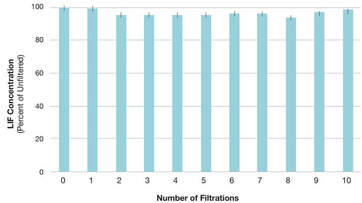
Figure 1. The retention of LIF in the complete mESC growth media following multiple filtrations using Nalgene™ Rapid-Flow PES filters.
