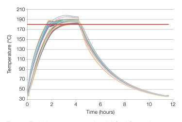
Figure 4. Typical temperature map for a full Steri-Run cycle. Thermocouples were placed in 48 locations in the chamber, including the walls, glass door, water reservoir cover and floor, and 3 shelves. All areas reached a minimum of 180°C. N =  $2 \times 4$  units.
