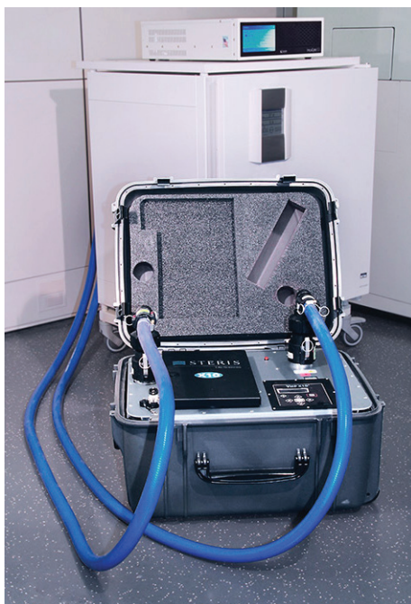
Figure 1: A Thermo Scientific™ Heracell™ 240i CO 2 incubator housing an Essen™ IncuCyte™ system is decontaminated using a biodecontamination system (Steris Life Sciences). Image courtesy of Essen BioScience Inc., a Sartorius company. (Used with permission.)
