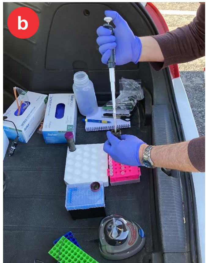
Figure 1 a) Sample homogenization and cell shearing onsite with a hand-held bead milling instrument, Figure 1 b) DNA extraction from sediment with Thermo Scientific mySpin 6 portable centrifuge in the boot of a car.
