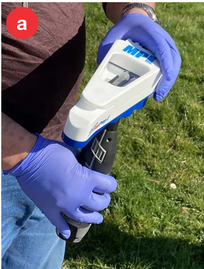
Figure 1 a) Sample homogenization and cell shearing onsite with a hand-held bead milling instrument, Figure 1 b) DNA extraction from sediment with Thermo Scientific mySpin 6 portable centrifuge in the boot of a car.
