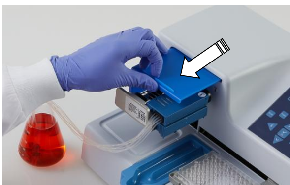
Figure 6-58. Pulling the rotor cover over the rotor
