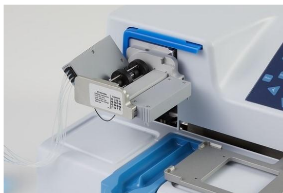
Figure 4-21. Rest position of the dispensing cassette
