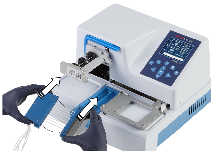
Figure 4-13. Inserting the dispensing cassette
