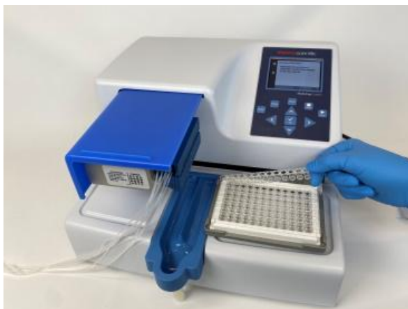
Figure 6-60. Removing the microstrip to be weighed
