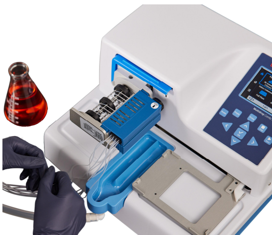
Figure 6-57. Dispensing cassette correctly installed
