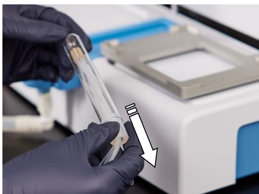
Figure 4–19. Removing the tubing weight protection and rubber holder
