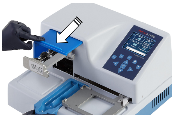
Figure 3–9. Pulling the rotor cover over the rotor
