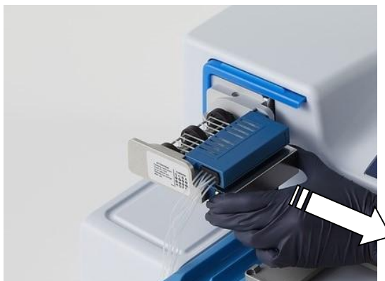
Figure 4–18. Pulling the tip protection off from the dispensing cassette
