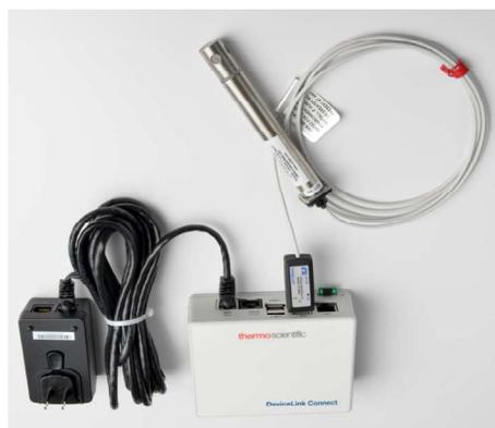
**Temp/RH Sensor Connected to DeviceLink Connect Mote**
