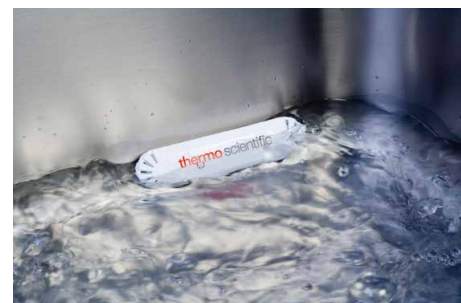
Figure 2. The Aqua-Tec Water Preservation Cell used in a water bath reservoir.
