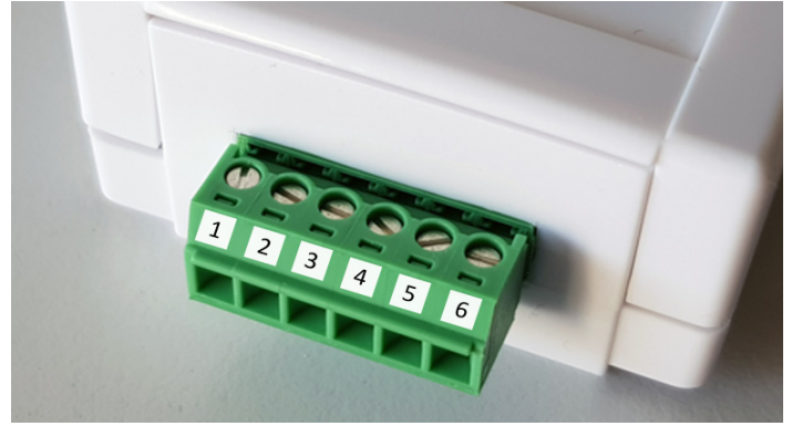
Figure 4. Smart Remote Contact Terminals
