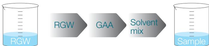
After titrations, remove the electrode from the sample and rinse it in this order, before soaking in RGW:
