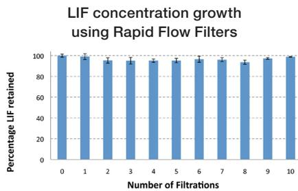
**Figure 1.** Filtration using Nalgene Rapid-Flow aPES filters did not significantly affect LIF concentration in mouse embryonic stem cell growth media.
