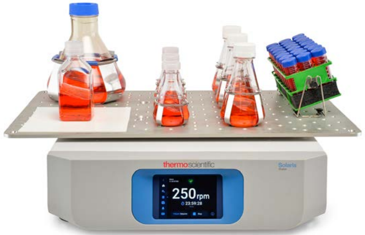
Figure 1: Different vessel types can be used on a shaker as long as they are balanced such that the weight is evenly distributed. If necessary, use a blank vessel as a counterbalance.
