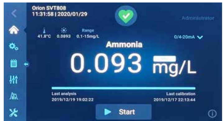
Figure 1. Intuitive touchscreen. With intuitive menu options that bring continuity across all process analyzers on the platform, the high-resolution interface displays standard icons and offers advanced diagnostics for ease of use and cross-training.
