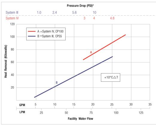
Facility water requirement is based on a 10°C difference between the temperature of the facility water supply and the application set point.
