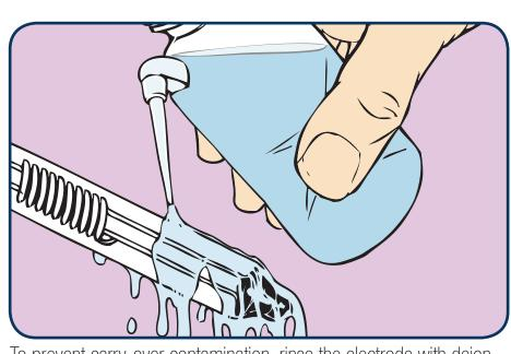
To prevent carry-over contamination, rinse the electrode with deionized water. Never wipe the electrode bulb as a resulting static charge may interfere with the accuracy of the test. Either blot the bulb gently and briefly with a lint-free laboratory wipe, or gently shake excess water drops from the end.
