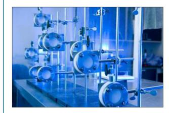
The test membrane was loaded into the test apparatus, then the bolts tightened to seal the perimeter. The test reservoir was filled with the bacteriophage challenge suspension and pressurized. Following the venting, the membrane surface was visually inspected for liquid penetration. Then each test reservoir was tested for the bacteriophage.
