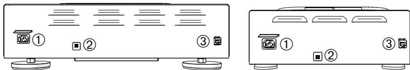
① Strømkobling; ② Sikring; ③ Ethernet-kontakt
