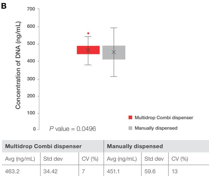
**Figure 2. DNA concentrations for DNA extracted from (A) plasma and (B) saliva samples using reagents dispensed manually or by the Multidrop Combi reagent dispenser.** Note the Student's *t*-test indicates that the average concentration of DNA is significantly different between dispensing methods for both types of samples.
