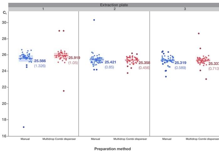
**Figure 4.**  $C_t$  values from the TaqMan RNase P Assay using gDNA from saliva samples treated with the SpecIMAX Stabilized kit and extracted with reagents dispensed manually or by the Multidrop Combi dispenser. Samples were extracted using the MagMAX DNA Ultra 2.0 kit.
