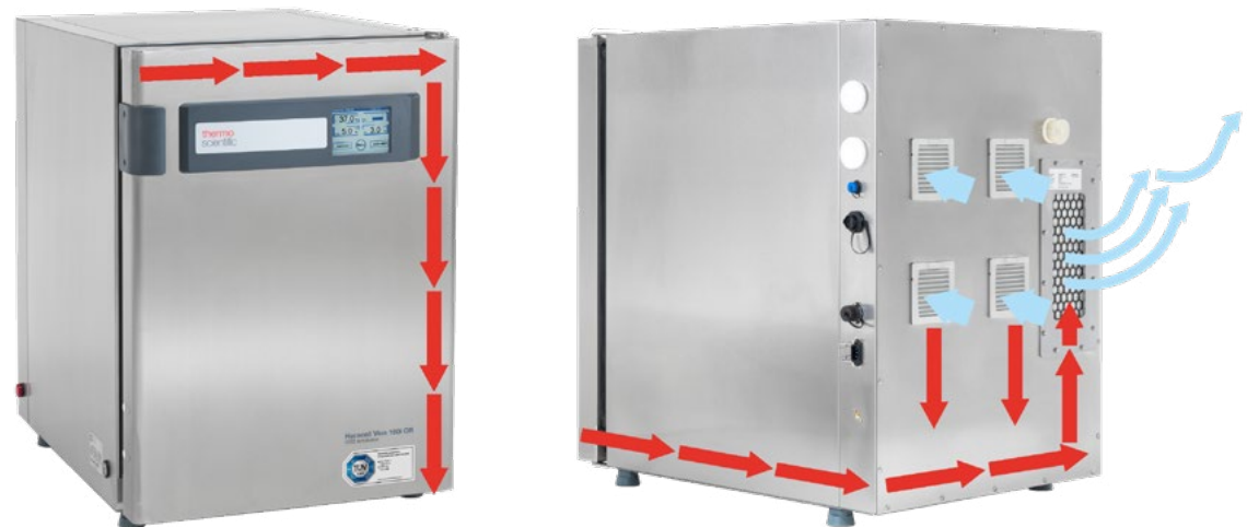
Figure 1. Active particle control system in a Heracell Vios CR CO 2 incubator collects particulates from the incubator casing and directs them to a HEPA filter in the rear wall. Incoming air from the cleanroom replaces the outgoing air.
