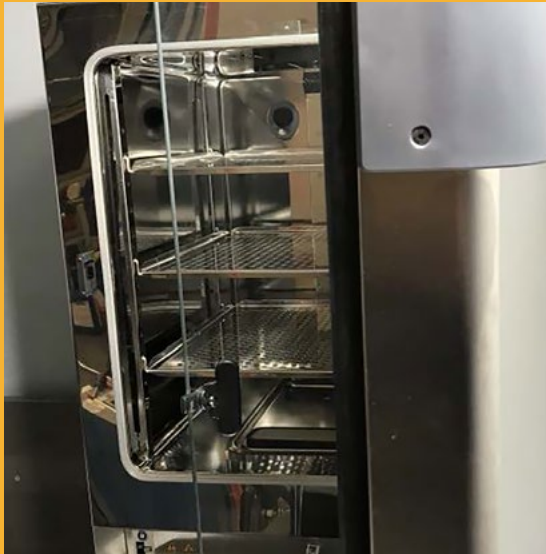
Figure 5. View of the front of a Heracell Vios 250i CR CO 2 incubator following sixteen cycles of 500 ppm STERIS VHP dry, non-condensing sterilization, showing complete compatibility with no negative effects.
