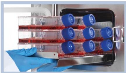
The non skid tray slides out to allow access to culture vessels, or the entire tray can be removed. The specialized design prevents tipping.
