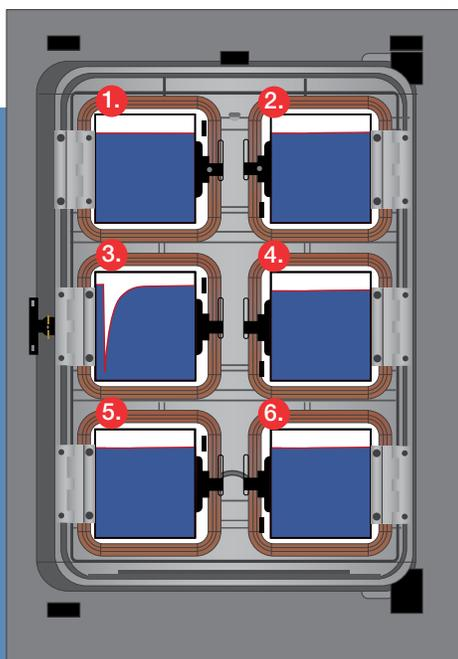
Demonstration of temperature, humidity and CO<sub>2</sub> stability in the unopened Cell Lockers when one Cell Locker (#3 as an example) is opened.
