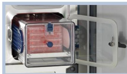
Remove the Cell Locker with optional transport cover to protect all cultures from outside air, for transport to a biological safety cabinet or to another lab.
