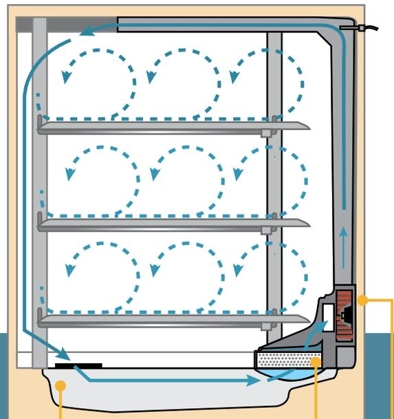
Incoming air first travels over a direct heated water reservoir resulting in 50% faster humidity recovery than with a standard water pan design.\*\*
