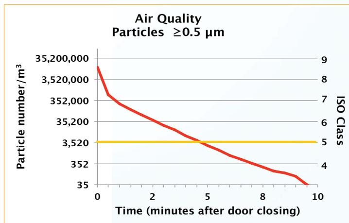
Our unique HEPA air filtration design reaches ISO Class 5 cleanroom air quality and recovers to that quality of air after a 30-second door closing within 5 minutes as tested in accordance with ISO 14644-1 and ISO 14644-3.
