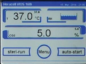
**New rH monitoring** assures the proper humidity level with indicator line icon. Low water alarm indicates critical low humidity levels requiring water addition.
