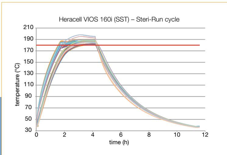
Validation that all surfaces reach 180°C with 48 point test on all chamber areas including the glass door and shelves.
