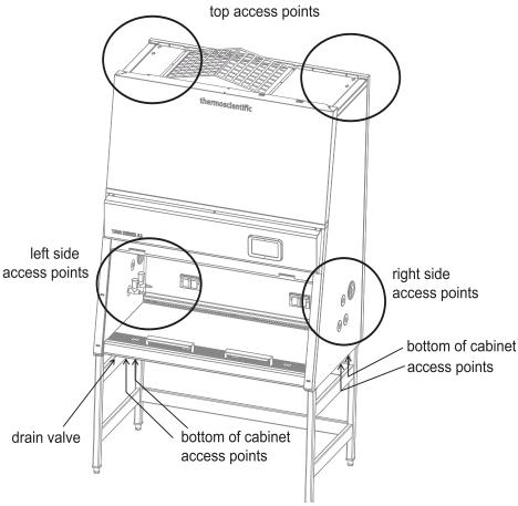
Figure 1-1. Unit Components
