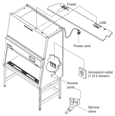
Figure 1-6. Interfaces (2 of 4 access ports are shown)
