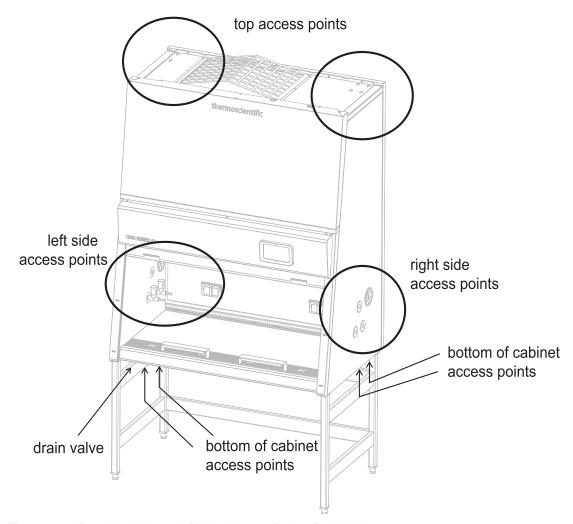
Figure 2-6. Possible Universal Piping Access Points/Drain Valve
