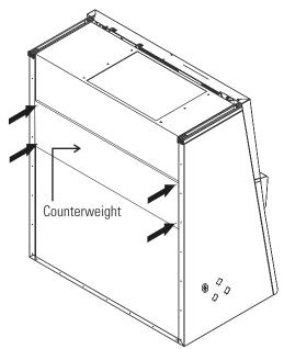
Figure 3-2. Unlocking the Counterweight
