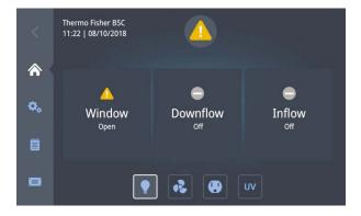
Figure 4-16. Main Screen - Unit in Idle Mode, window opened
