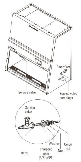
Figure 2-5. Valve Assembly and Installation
