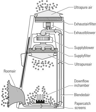
Figure 1-2. Airflow Filtering System
