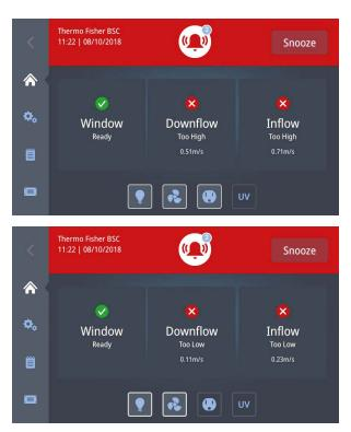
Figure 4-23. Alarming Screen for Downflow too high and too low Alarm
