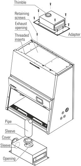
Figure 2-2. 6 ft Thimble and Sleeve
