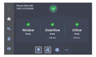
Figure 4-12. Main Screen - Unit working
