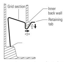
Figure 5-1. Protective Paper Catch Grid
