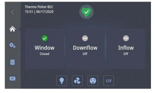
**Figure 4-5.** Main screen — Unit in Idle Mode
