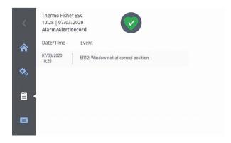
Figure 4-32. "Alarm/Alert log" Logfile Screen
