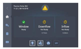
Figure 4-11. Main Screen - Unit starting up
