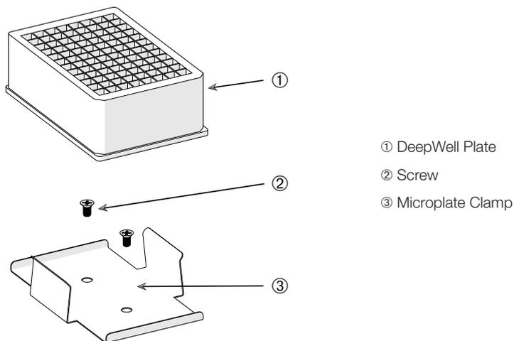
**Figure 86:** Microplate / DeepWell-plate Clamp Assembly
