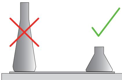
**Figure 95:** Adhesive Mat: Suitable Flask Shapes
