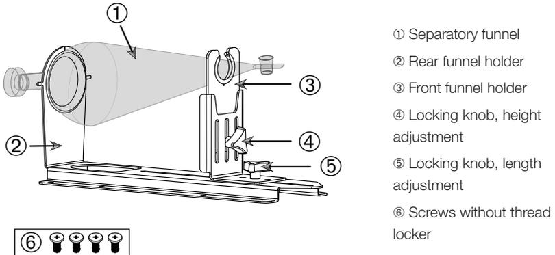
Figure 92: Separatory Funnel Clamp Assembly
