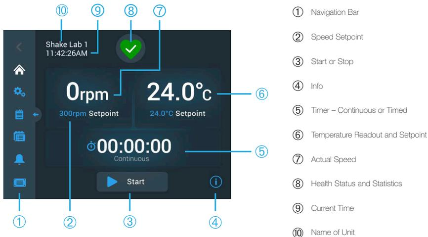
Figure 27: GUI Home Screen for Temperature Controlled Shaker
