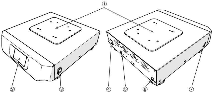
① Platform Mounting Plate; ② Graphical User Interface (GUI); ③ Power Supply Switch; ④ Mains Connection; ⑤ Fuse (resettable); ⑥ Ethernet Port; ⑦ USB Port
