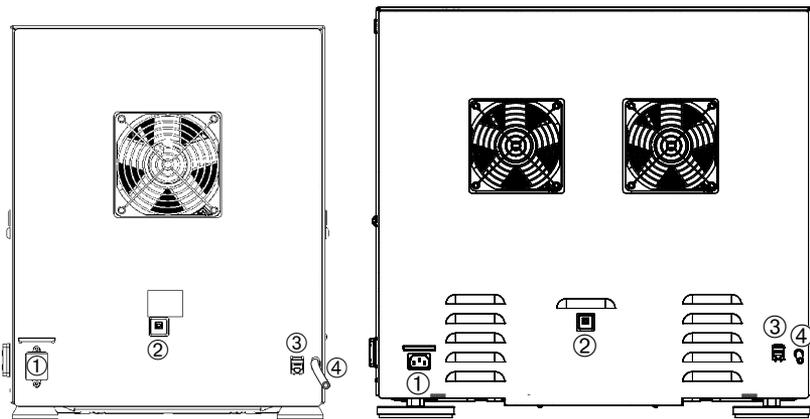
① Mains Connection; ② Fuse; ③ Ethernet Port; ④ Drain Tube
