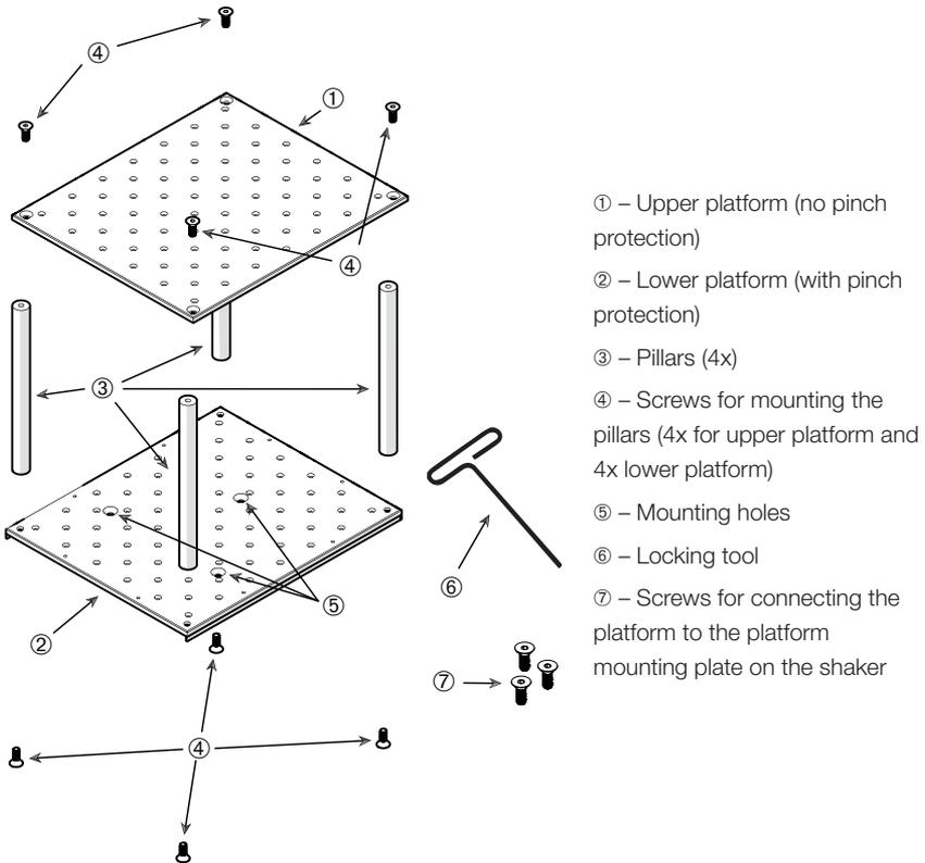
**Figure 79:** Dual Stack Platform Assembly
