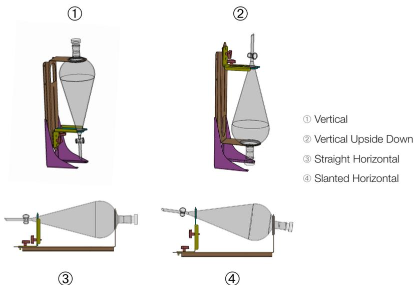
**Figure 90:** Separatory Funnel Clamp Mounting Positions
