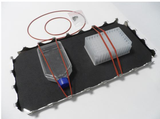
Figure 94: Utility Tray with Containers Installed and O-Rings
