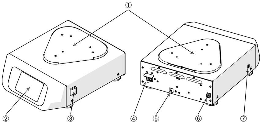
① Platform Mounting Plate; ② Graphical User Interface (GUI); ③ Power Supply Switch; ④ Mains Connection; ⑤ Fuse; ⑥ Ethernet Port; ⑦ USB Port
