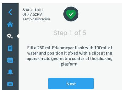
Figure 108: Calibration: Prompt for filling Erlenmeyer flask
