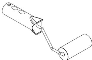
Figure 96: Rolling Applicator for Adhesive Mat
