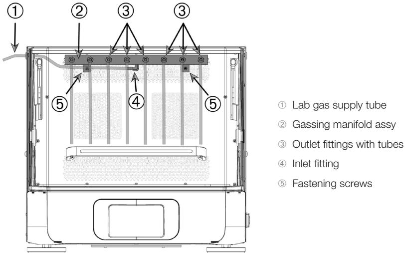
Figure 100: Gassing Manifold Installed in Solaris 4000 R Shaker
