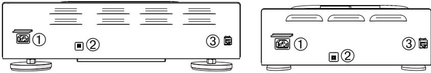
① Mains Connection; ② Fuse; ③ Ethernet Port
