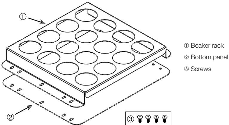
**Figure 89:** Beaker Rack Assembly
