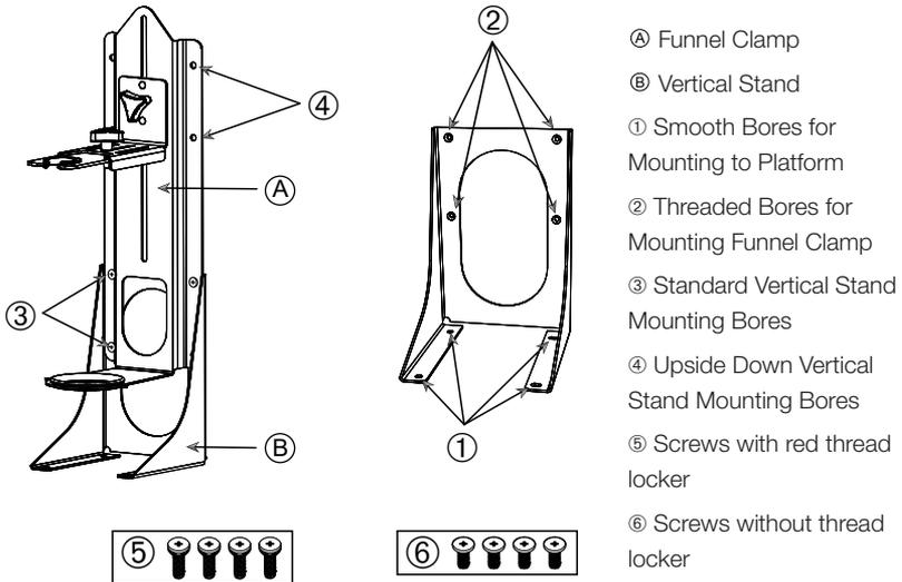
Figure 91: Separatory Funnel Clamp (right) with Vertical Stand Accessory (left)
