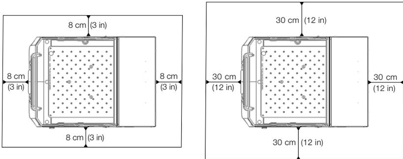
**Figure 9:** Set Up Clearances for Incubated (left) and Refrigerated Shakers (right); refrigerated with free air above are covered by the left image.
