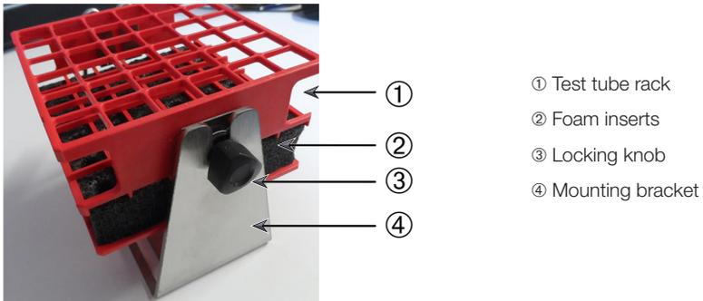
**Figure 84:** Test Tube Rack Assembly with Sheet Metal Mounting Bracket
