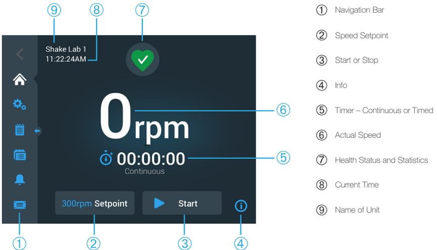
Figure 26: GUI Home Screen for Open Air Shaker
