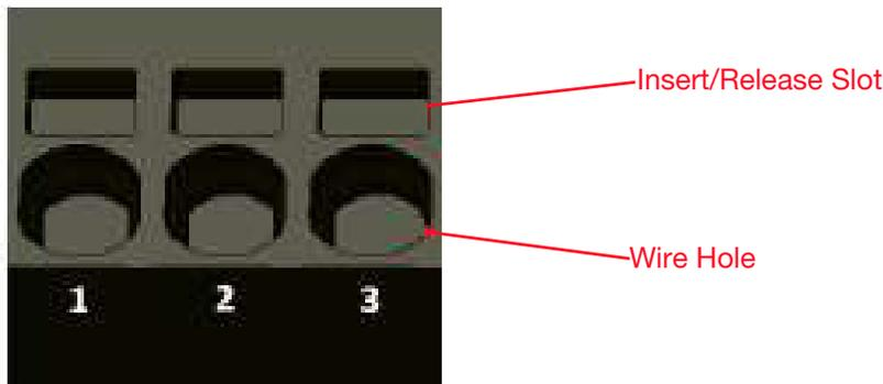
Figure 18. Smart-Cable terminal block (RTD shown)
