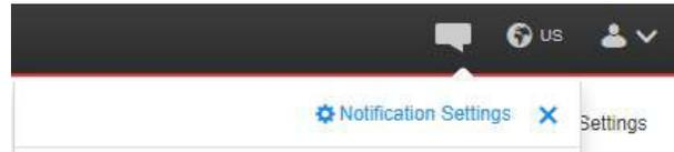
Access the notification settings window by clicking on the Notification icon at the top-right of the InstrumentConnect window. These settings apply globally to all instruments a specific user is connected to.
