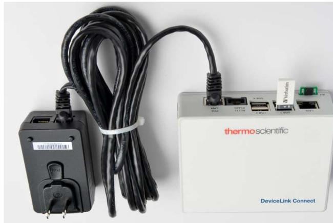
**Figure 2. Connecting Supply power to DeviceLink Connect mote**
