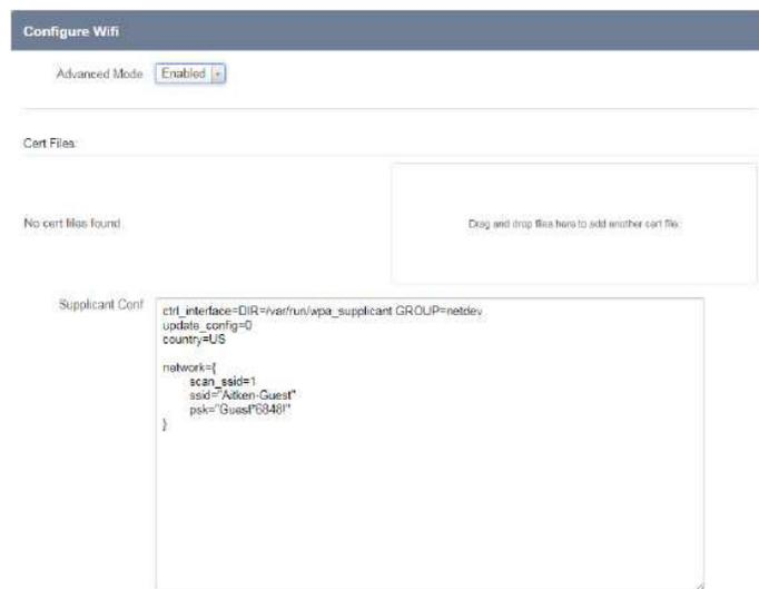
**Figure 21. Configuring Wi-Fi advanced mode**
