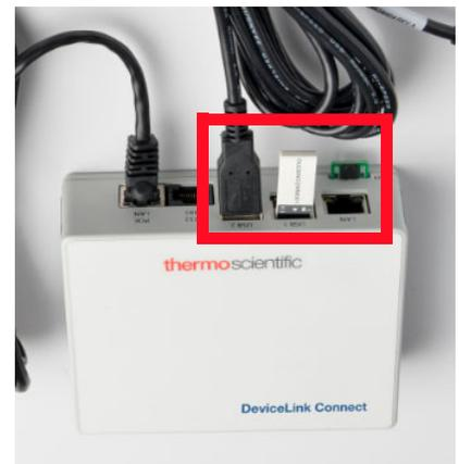
**Figure 3. Installing USB Commissioner dongle to DeviceLink Connect mote**
