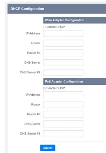
The screenshot shows the "DHCP Configuration" form. Under "Wlan Adapter Configuration", the "Enable DHCP" checkbox is unchecked, and fields for "IP Address", "Router", "Router #2", "DNS Server", and "DNS Server #2" are visible. Under "PoE Adapter Configuration", the "Enable DHCP" checkbox is also unchecked, and the same set of fields is visible. A blue "Submit" button is at the bottom.
