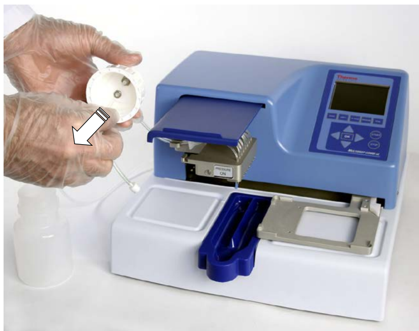
Figure 5–27. Removing the reagent filter with tube
