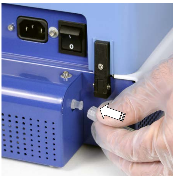
Figure 3–10. Connecting the hosing to the pressure/vacuum system
