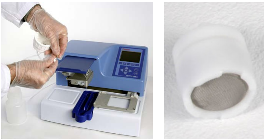
Figure 4-18. Removing the reagent filter
