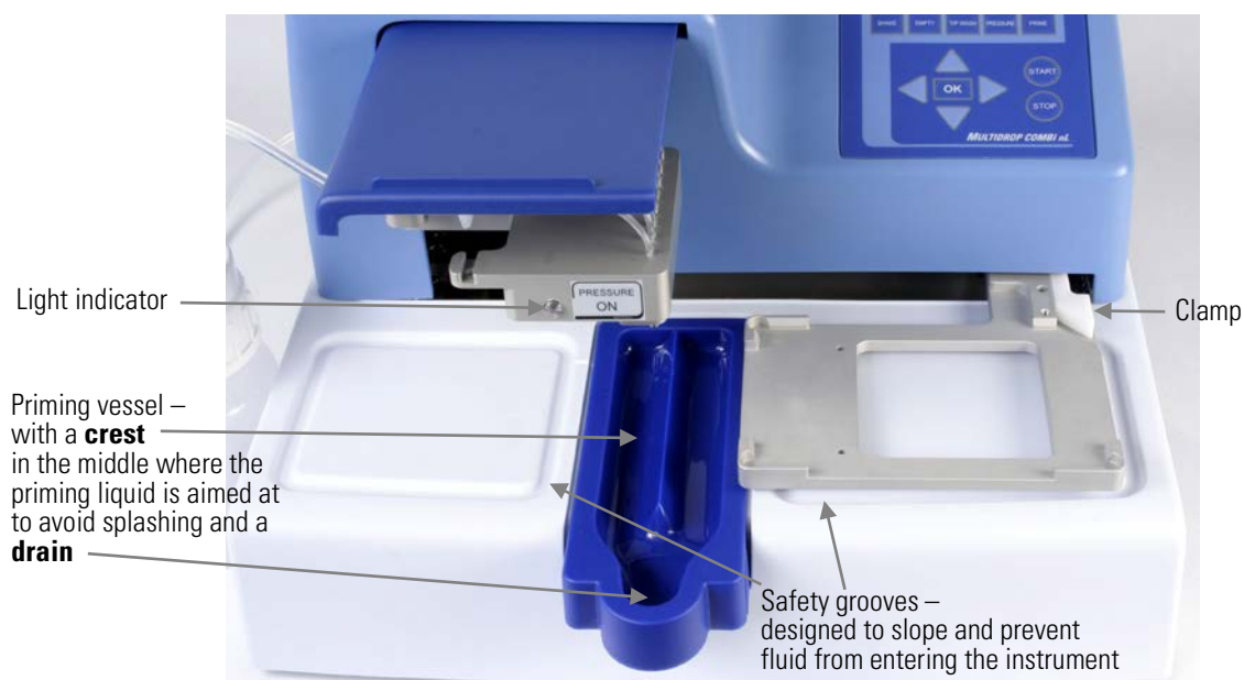
Figure 3–14. Priming vessel inserted into place
