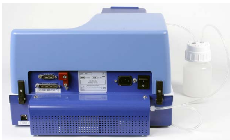
Figure 3–7. Transport lock storage
