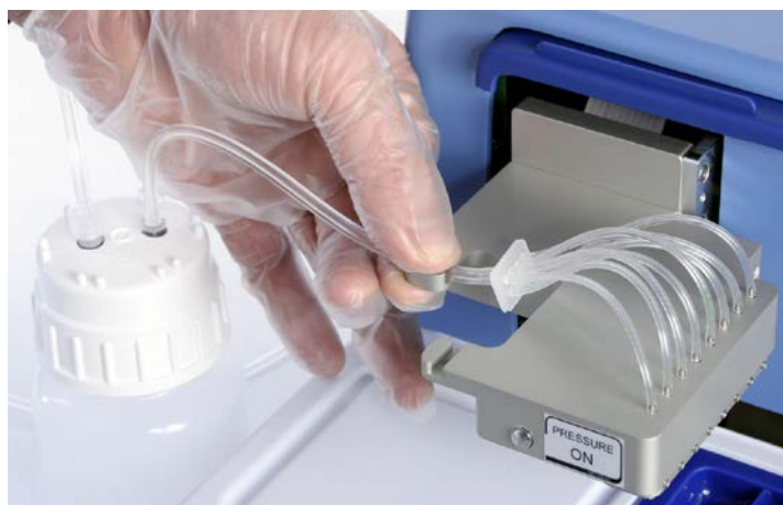
Figure 5–31. Replacing the tubing set and manifold
