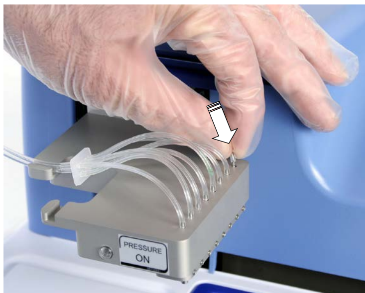
Figure 5–26. Reconnecting a dispensing valve tube end
