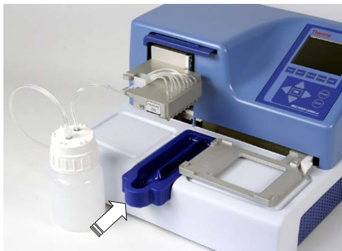
Figure 3–8. Inserting the priming vessel
