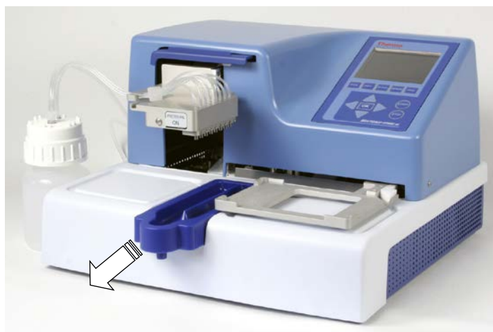
Figure 5-32. Unfastening the priming vessel
