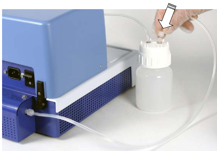
Figure 3-11. Connecting the hosing to the reagent reservoir
