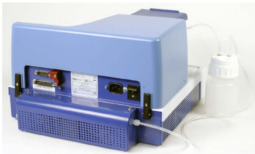
Figure 5–33. Transport lock storage location
