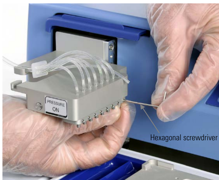
Figure 5–28. Unfastening the dispensing valve
