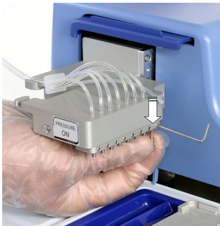
Figure 5–29. Pulling the dispensing valve downwards
