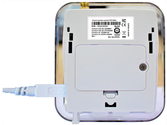
Figure 74. Optional: plug data logger into AC (USB) power to avoid losing data
