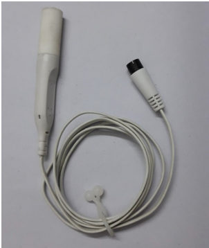
Figure 27. Dual temperature-humidity sensor
