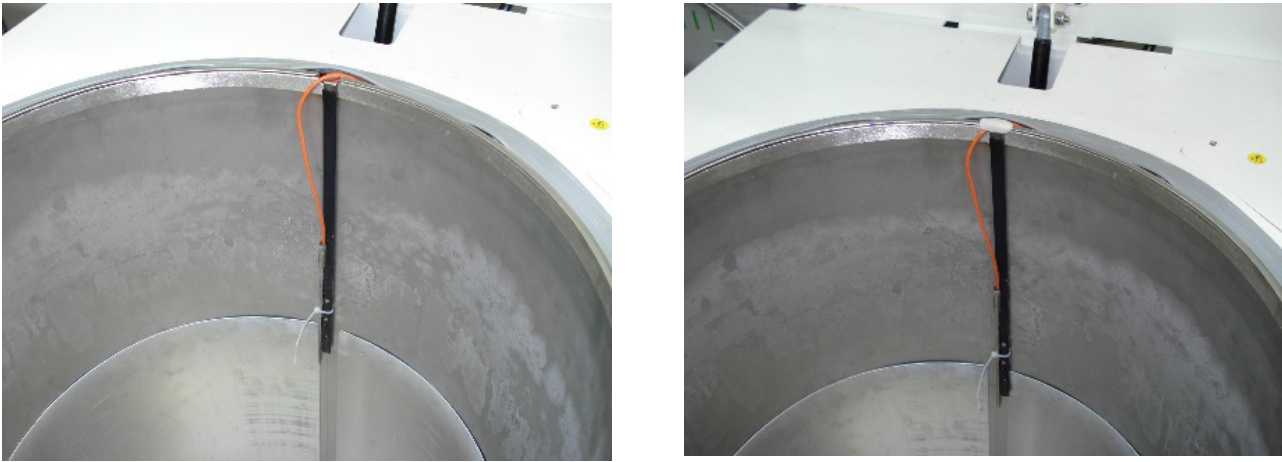
Figure 22. Pt100 (-200 °C to + 50 °C) for nitrogen/cryogenic tank
