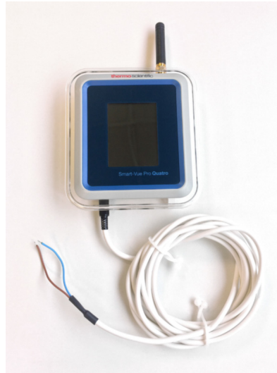
Figure 28. Smart-Vue Pro Duo/Quatro with dry contact input cable
