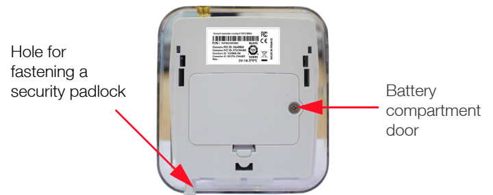
Figure 5. Rear view of the data logger
