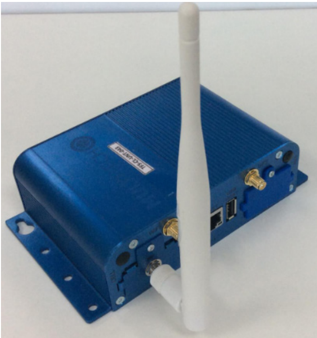
Figure 3. Attach Smart-Vue Pro LoRaWAN Antenna to connector labeled “RF”
