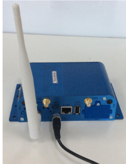
Figure 4. Plug in the power cable to the stainless steel connector
