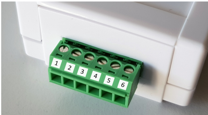
Figure 4. Smart Remote Contact Terminals
