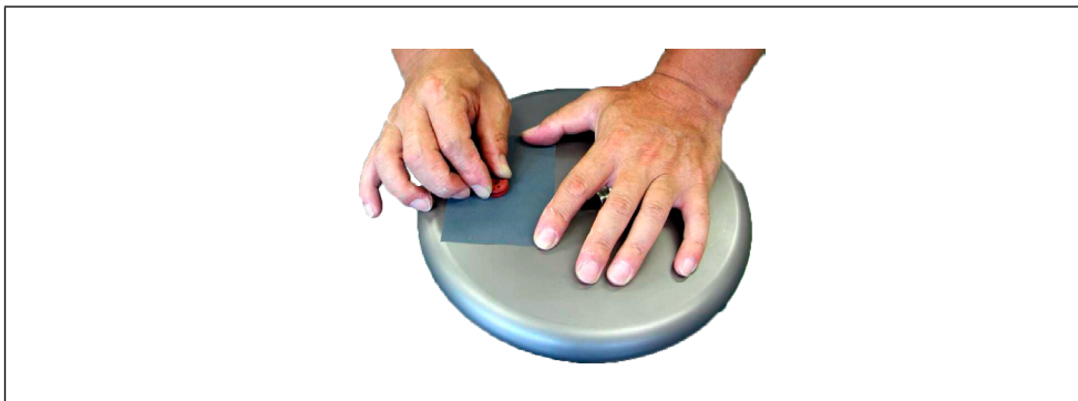
Figure 41 Polishing the Rulon seal
