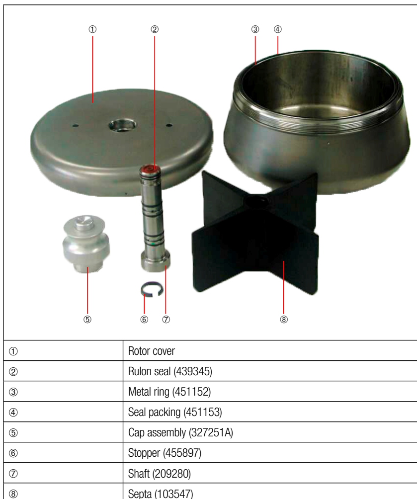
Figure 1 Rotor Components
