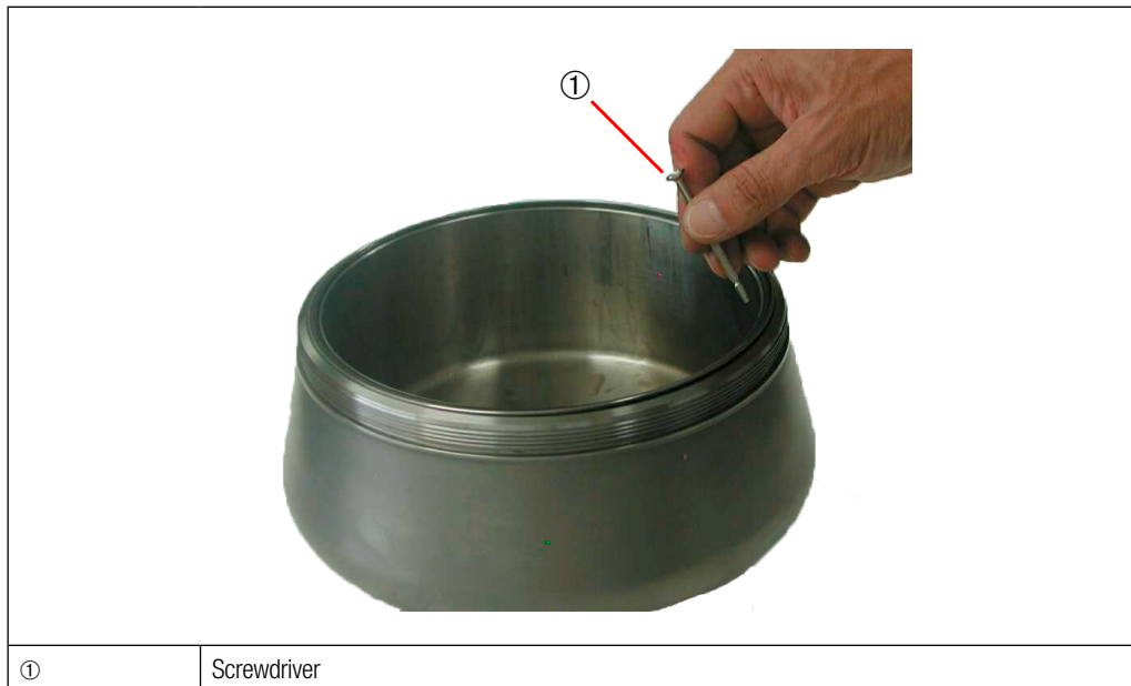
Figure 39 Removal of the metal ring
