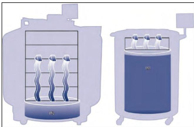
**Figure 2. Illustration showing LN<sub>2</sub> as the refrigerant.**
