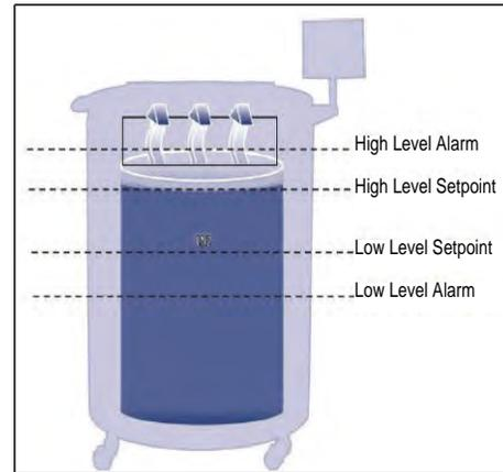
**Figure 4. Example of automatic level control parameters**
