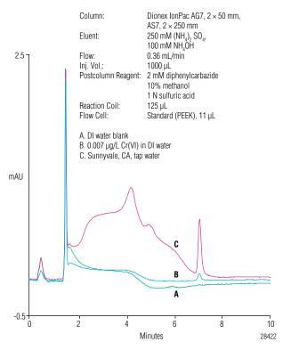
Figure 3. Determination of Cr(VI) in A) DI water blank, B) 0.007  $\mu$ g/L, and C) Sunnyvale, CA, tap water blank on a Dionex ICS-3000 system. Postcolumn reagent delivered by the second pump of DP. Flow cell: standard (PEEK).
