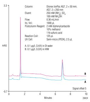
Figure 5. Determination of Cr(VI) (0.1  $\mu$ g/L) in A) DI water and B) HIW on an ICS-2100 system. Postcolumn reagent delivered by an AXP pump. Flow cell: semi-micro (PEEK).
