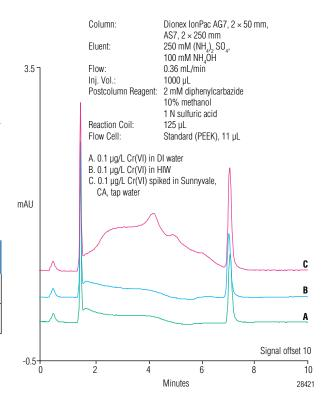
Figure 2. Determination of Cr(VI) in A) DI water, B) HIW, and C) Sunnyvale, CA, tap water using a Dionex ICS-3000 system. Sunnyvale, CA, tap water blank has a background Cr(VI) level of 0.05  $\mu$ g/L Cr(VI). Postcolumn reagent delivered by an AXP pump. Flow cell: standard (PEEK).
