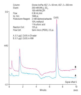
Figure 1. Determination of Cr(VI) (0.1  $\mu g/L$ ) in A) DI water and B) HIW on a Dionex ICS-3000 system. Postcolumn reagent delivered by a DP pump. Flow cell: semi-micro (PEEK).
