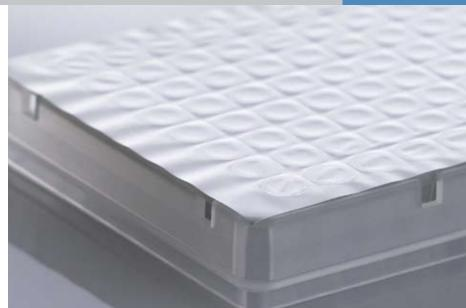
Quality Sealing Options. With the semiautomated Thermo Scientific ALPS 50 V microplate heat sealer, secure tight seals around individual wells to eliminate sample loss through evaporation and cross contamination between wells. Choose from a wide range of heat seals, including piercable, optically clear and permanent, for any application.
