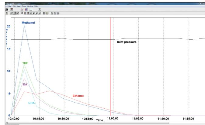
Figure 2: One dryer containing 5 solvents, the other containing just one solvent. Note that all other solvent readings remain at zero in dryer 2
