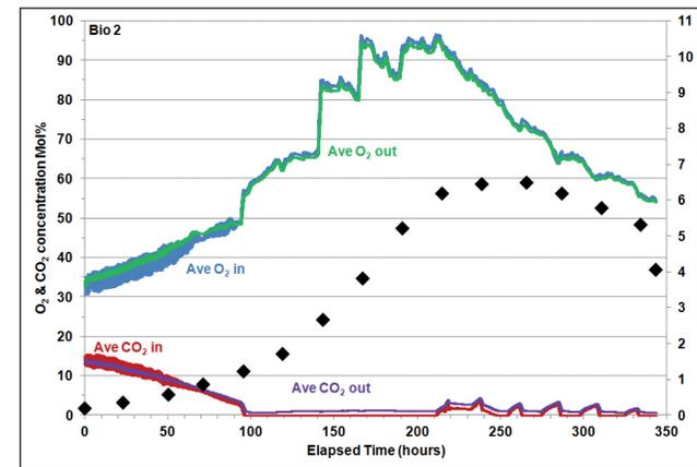
**Figure 1:** Online MS gas concentration data and offline VCC data from two mammalian cell bioreactors
