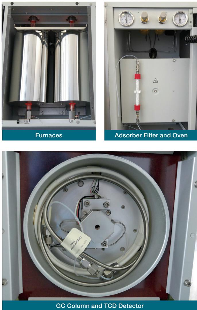
Figure 4. FlashSmart CHN and Oxygen internal circuits.
