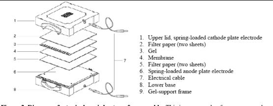
**Figure 2. Diagram of a typical semi-dry transfer assembly.** This is an example of a non-powered blotter whose electrical cables must be connected to a power supply. Newer devices, such as the Pierce G2 Fast Blotter (Part No. 62288), have integrated cassette and power control units that provide convenience and optimal performance for rapid transfer protocols.
