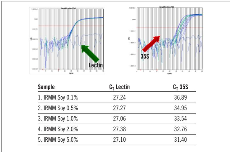
**Figure 4.** Real-time PCR analysis (using a 7900HT system and the 5' nuclease assay) for the lectin and 35S genes in DNA, isolated from IRMM reference materials (using a 6100 PrepStation and TransPrep chemistry).
