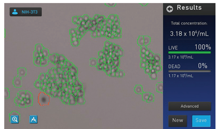
Figure 3. Accurate cell counts, even with clumpy samples. The segmentation and counting algorithms of the Countess II cell counters are able to resolve clumps of cells in this NIH/3T3 cell sample.
