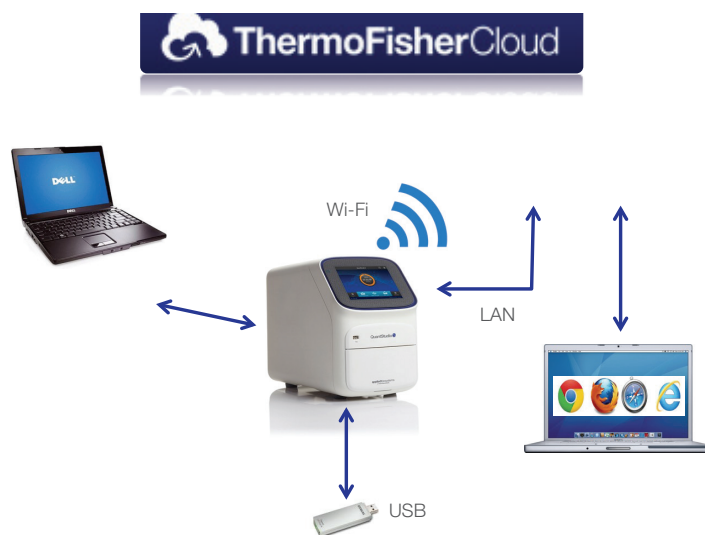
Figure 1. QuantStudio 3 and 5 Real-Time PCR System connectivity: stand alone, desktop, or online. The QuantStudio 3 and 5 systems can connect by laptop to the QuantStudio Design and Analysis Software. The systems can also connect to the QuantStudio Design and Analysis Software on Thermo Fisher Cloud using any device with a web browser. The system may also be used as a stand-alone instrument, with data transfer by USB or Wi-Fi connection to the web browser-based software.
