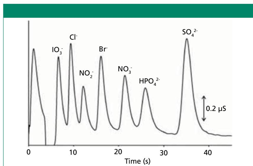
**Figure 3:** Ultrafast separation of seven common anions on very short column (1.3 cm × 0.46 cm) with suppressed conductivity detection. Column: Cationic surfactant (didodecylmethylammonium bromide) coated Extend-C18 column; flow rate: 2.0 mL/min; particle size: 1.8  $\mu$ m; eluent: 2.5 mM 4-hydroxybenzoic acid (pH 10.1). Adapted from reference 20.
