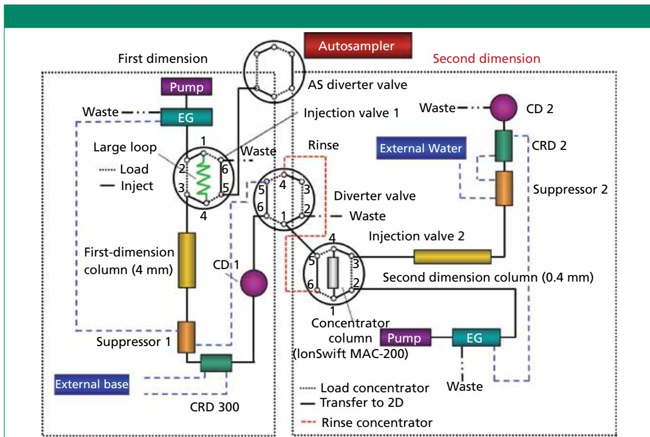
**Figure 3:** Two-dimensional ion chromatography instrumental setup.
