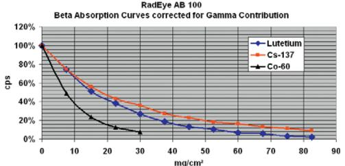
Absorption measurements show that the beta emission spectrum is right between Cs-137 and Co-60. The calculated effective maximum beta energy of the thick  $Lu_2O_3$  layer is approximately 480 keV.
