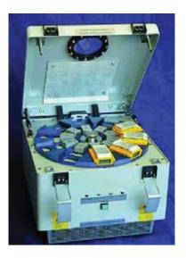
A carousel holding up to 10 EPDs, either Mk1 or Mk2 but not mixed, is loaded onto the IRR-2. On starting the cycle, all dosemeters are status-checked before irradiation commences. On completion of each EPD irradiation the dose and counter data is uploaded to EMDS2 which can run on the same PC as the Auto Irradiator software. Here the data is compared with preprogrammed limits and any historical data in the database for individual EPDs.
