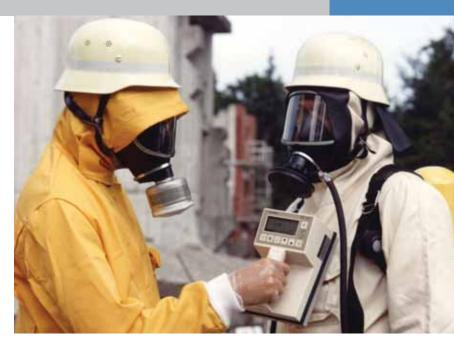
The Contamat performs alpha and beta/gamma contamination measurements. Separate alpha and beta/gamma alarm values are monitored simultaneously. The measurement results are displayed in analog and digital form in s¹, Bq or Bq/ cm². In counter mode, the elapsed measurement time is displayed in addition to the measured value. Accuracy of measurement can be checked by push-button.
