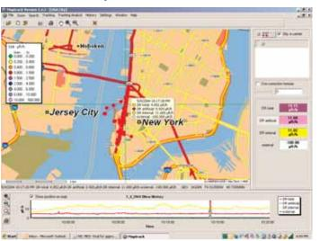
The exclusive MAPTRACK program is a global positioning based movable mapping system that automatically records radiation measurement data along the path of travel. It utilizes a 6 channel Global Positioning System (GPS) to closely track the exact coordinates. The MDS is sold with a GPS antenna. But MAP-TRACK can accommodate any type of GPS if a particular type of GPS system is required.
