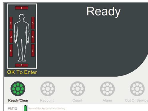
Along with these indicators, a human silhouette, located on the right hand side of the portal frame, indicates which of the eight detector zones are “contaminated” thus aiding in localizing the contamination on an individual. The monitor will utilize double detector and triple detector sum-zones for monitoring of low level distributed activity. Voice commands may be utilized to help with the positioning of the user.
