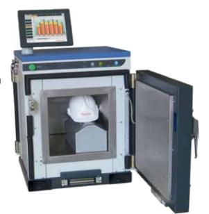
Articles used in radiation controlled areas of nuclear facilities should undergo monitoring to confirm they are free of contamination. In the US, this clearance limit is 5000 dpm, which is easily achievable by the SAM12 for higher energy gamma emitters such as Cs-137 and Co-60.
