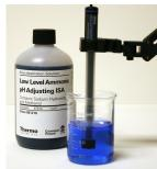
Sample with Ammonia ISA Solution Added Color Changing Blue Dye Indicates Correct Sample pH for Ammonia Measurements
