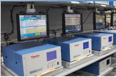
The Thermo Scientific Calibrator Certification Service compares and validates the Thermo Scientific Model 81*i* Mercury Calibrator to a NIST (National Institute of Standards and Technology) traceable Vendor Prime or Field Reference Generator. The calibration method is based on the Interim Draft Traceability Protocol as set forth by NIST and the Environmental Protection Agency (EPA).
