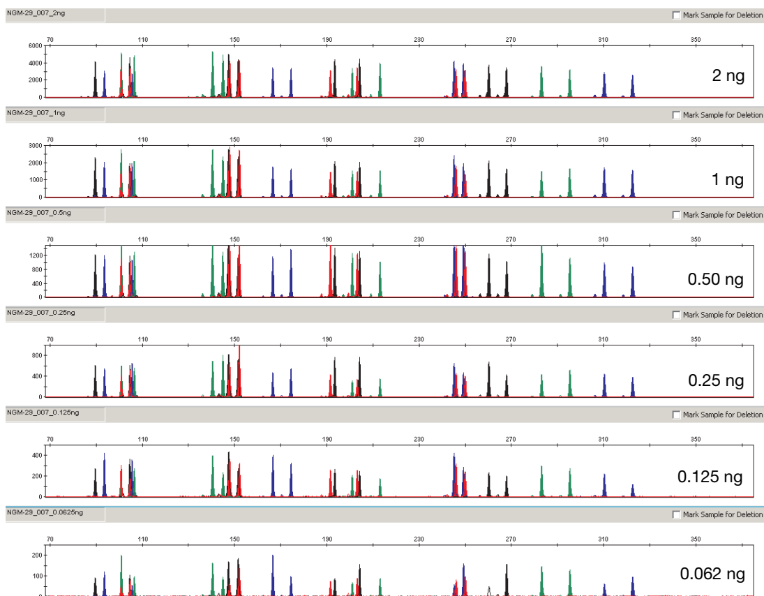
Figure 31 Electropherograms for amplifications using 2 ng, 1 ng, 0.50 ng, 0.25 ng, 0.125 ng, and 0.062 ng of control DNA 007. Electrophoresis was performed on an Applied Biosystems 3130xI Genetic Analyzer. Note that the y-axis scale is magnified for the smaller input amounts of DNA.
