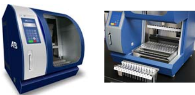
Figure 1. Bench top AutoMate Express™ System using PrepFiler Express™ and PrepFiler Express BTA™ Forensic DNA Extraction kits.
