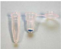
Figure 2. PrepFiler LySep™ column was developed to provide effective one-step lysis and separation of large size particulate from lysate without any manual transfer steps.
