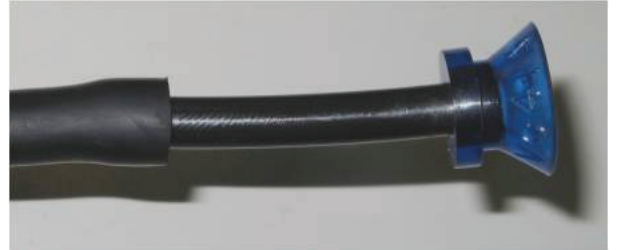
Figure 6. Leak check adapter installed in sample line.
