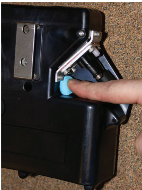
Figure 5. Placing the leak check putty in pump exhaust port opening.
